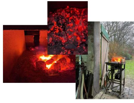
The cutting tools are traditionally forged. The material used is spring steel from discarded carts. The molecular structure of the steel is broken under heat. The steel, softened for a brief moment, can be deformed under the force of hammer blows. Through corresponding expulsion, the blade is compacted. The steel is then tempered in grease and rehardened in the fire.
