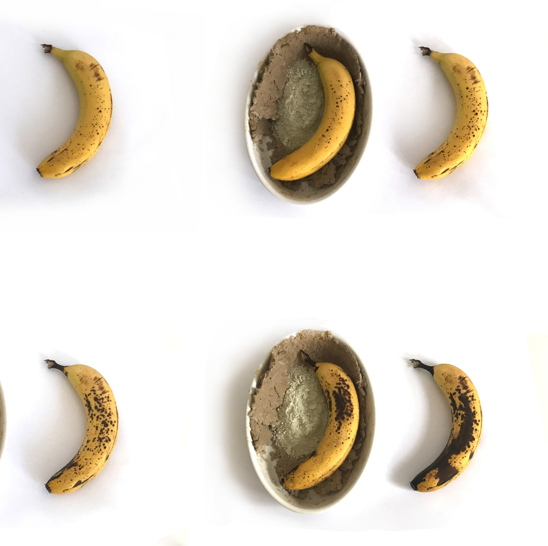
ripening process of two bananas over the course of 10 days, one in contact with zeolite , one without.
