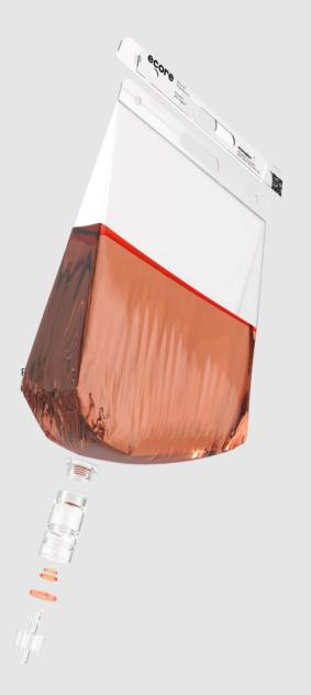
Radio-sonic welds shape the volume and connect the top handle as well as the thread port. The information of the top handle is laser engraved and thus does not add any contaminant to the material.
