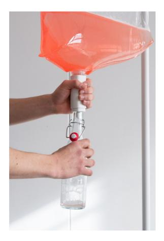
To ensure convenient usability and meet the demands of a mono-material design, the dispenser, just as the bag and handle, uses the versatile properties of Elastollan<sup>®</sup>, serving a wide range of Shore hardnesses from very soft and flexible to hard and springy. It consists of a housing screwed to the bag, a movable trigger, a corresponding disk spring and two sealing rings.
